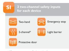
\*Option to connect 2-channel safety transmitters (such as speed monitors, standstill monitors, ...)
