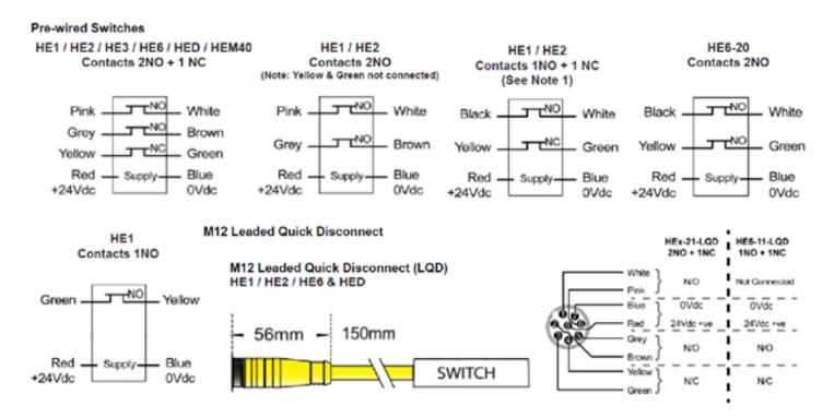
CONTACT OPERATION -The N/O contact(s) on Mechan safety switches are open when the actuator is away from the switch. When the actuator is within the specified operating distance the N/O contact(s) will close and the N/C contact will open
