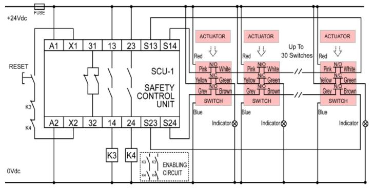
NOTE 1 : THE SCU-1 SAFETY CONTROL UNIT IS DESIGNED TO WORK WITH 2 X NO INPUT FROM THE HE SAFETY SWITCHES
