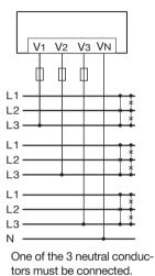
Fig.: Voltage measurement in up to three symmetrically load-ed three-phase 3-conductor systems (only UMG 96-PA, not UMG 96-PA-MID+)
