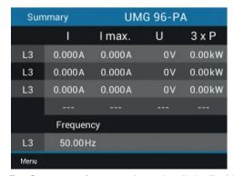
Fig. Start screen for connection variant 3p1w (3 x L3)
