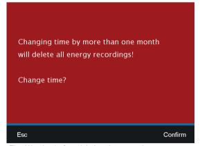
Fig. Warning before deleting data records
