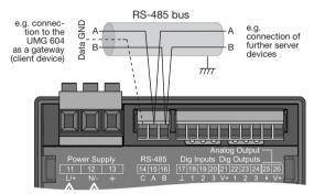
Fig. RS-485 interface, 3-pole plug contact
