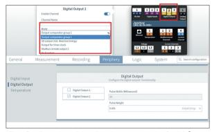
Fig. Configuration of the digital outputs via the GridVis® software
