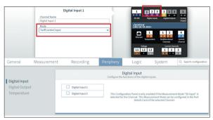
Fig. Configuration of digital input 1 as a tariff control input in the GridVis ® software
