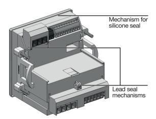
Fig. Rear view of the measurement device with terminal covers, lead seal mechanisms and the mechanism for the silicone seal.
