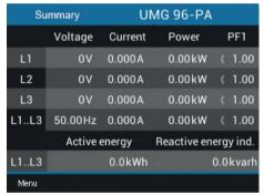
Fig. Measuring display "Overview" - measurement in a three-phase four-wire network (default setting).
