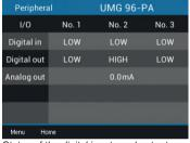
States of the digital inputs and outputs, value of the analog output
