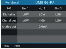
Fig. Displays the states of the digital inputs and outputs and the value of the analog output.
