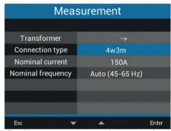
Fig. Measurement window with the entries for the transformers
