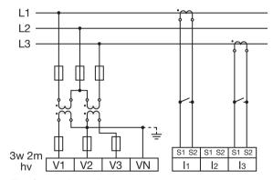
Fig. Connection variant 3w2m hv - measurement via 2 voltage transformers in a three-phase 3-conductor network with asymmetrical load.
