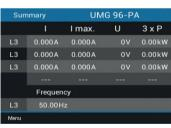
Symmetrically loaded networks 3 x L3 (3p1w. only for UMG 96-PA, not UMG 96-PA-MID+):
