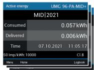
Displays sum (L1..L3) of active energy according to MID, reactive and apparent energy
