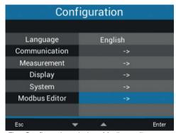
Fig. Configuration window, Modbus editor
