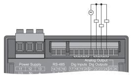
Fig. Connection of digital/pulse outputs
