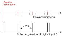
Fig. Principle of synchronization with "periodic pulses" to digital input 3
