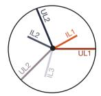
Current and voltage are shifted against each other. The current is ahead the voltage, i.e. the network is capacitively loaded.
