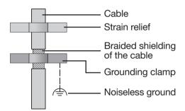
Fig. Shielding design for cabinet entry.
