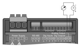
Fig. Analog output connection
