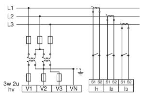
Fig. Connection variant 3w2u hv - measurement via 2 voltage transformers in a three-phase 3-conductor network with asymmetrical load.
