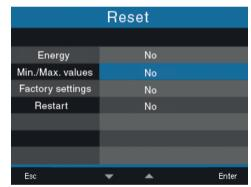
Fig. Reset window, delete min/max values
