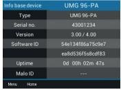
Device type, serial number, firmware version, software ID, running time (since last power-on or software reset) and market location ID
