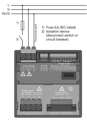
Fig. "Supply voltage" connection example
