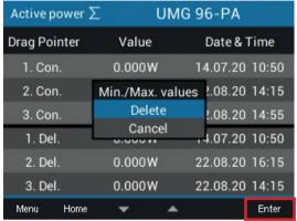
Fig. Dialog box for deleting the drag indicator values
