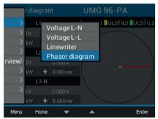
Fig. Submenu item Phasor diagram
