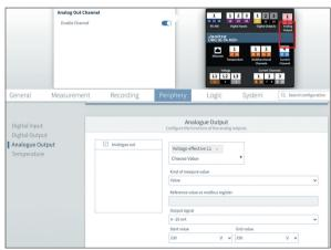
Fig. Configuration of the analog output in the GridVis <sup>®</sup> software
