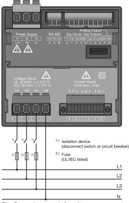
Fig. Connection example for voltage measurement.
