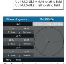
Fig. Phasor diagram window showing the phase sequence according to the direction of the rotary field
