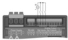
Fig. Connection of digital inputs
