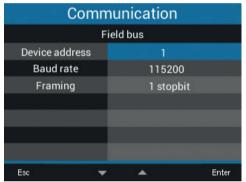
Fig. Communication window for fieldbus parameters (RS-485 interface)
