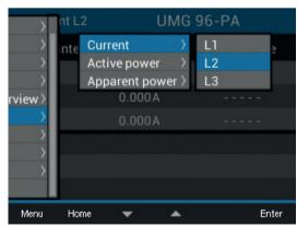
Fig. Drag indicator display with the submenu items Current, Active power and Apparent power.
