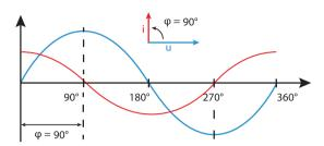
With a combination of the states, the phase angle "current to voltage" can assume values between -90° and +90°.
