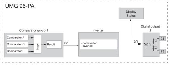
Fig. Block diagram "Using digital output 2 for limit value monitoring"
