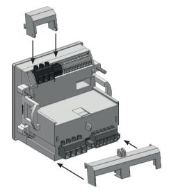
Fig. Installation of the terminal covers on the measurement device
