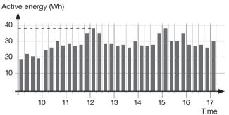
Consumption measurement 12:00 hrs: 558 Wh Consumption measurement 11:45 hrs: 520 Wh Difference: **38 Wh**
