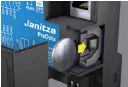
Fig.: Easy replacement of the battery during operation
