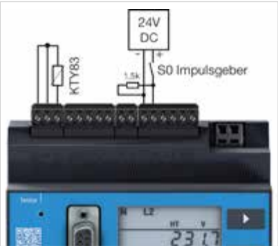
Fig.: Example thermistor input (KTY83) and S0 pulse generator
