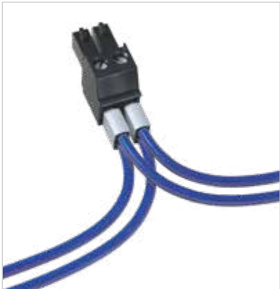
Fig.: 2-pole plug contact with cable connection (cable type: 2 x 0.75 mm 2 ) via twin wire ferrules
