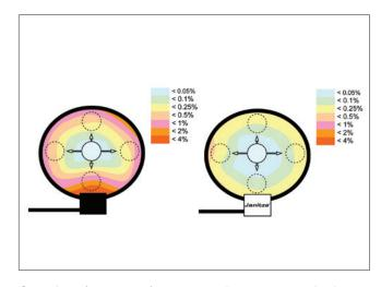
Comparison of current transformer accuracy between a conventional Rogowski current transformer and the patented Janitza solution with consideration to the installation position
