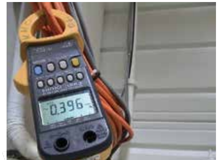
Fig.: Avoidance of stray currents on data lines
