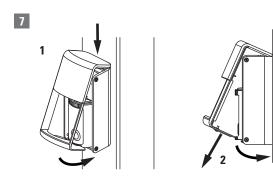
First hook the front cover on the top of the base and then snap it onto the base while pulling down.
