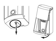
Loosen the retaining screws on the bottom of the front cover and remove the front cover.
