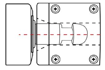
Ensure the actuator plunger and targets are correctly aligned.
