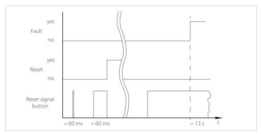
If the actuation period is not reached, then reset will not take place. If the actuation period max. is exceeded, the control unit changes to the mode: "Fault / System error" (see Chapter *Troubleshooting and remedies*).
