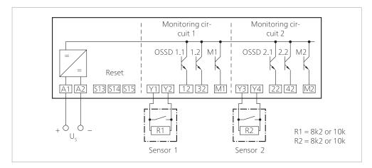
The OSSDs 1.1, 1.2, 2.1 and 2.2 are semiconductor outputs (PNP) and short-circuit-proof. In the HIGH state (ON state) the voltage  $U_s$  -3 % tolerance is applied, depending on the voltage load and supply voltage.
