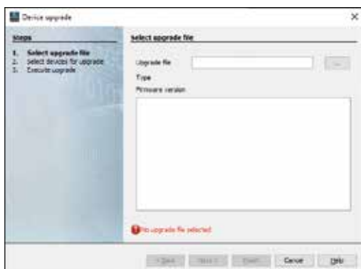
Fig. Updating the device firmware in the Grid Vis® software
