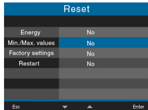
Fig. Reset window, delete min/max values
