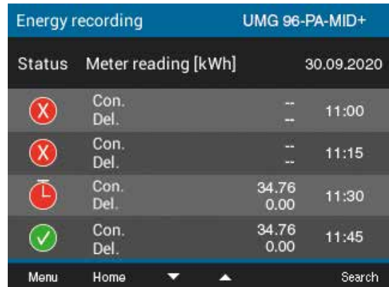
Fig. Example "Meter reading cycle" window with different symbols in the status (the time for recording the meter reading cycle was started between 11:30 and 11:45, on 09/30/2020).
