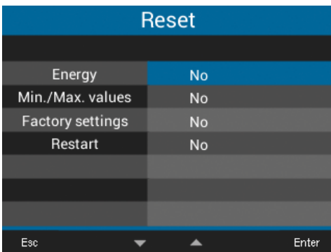
Fig. Reset window, resetting the energy meters
