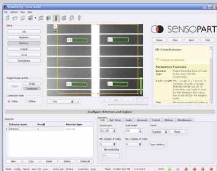
The easily comprehensible user interface of the VISOR® Code Reader Solar. In this live image it can be seen that all four ECC200 data matrix codes have been successfully read in one throughput.
