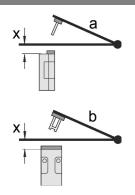
The axis of the hinge should be x mm above the top edge of the safety switch and in the same plane. a = Actuating radius to the plane of the actuator <math>b = Actuating radius in line with the plane of the actuator <math>x = Axial misalignment
